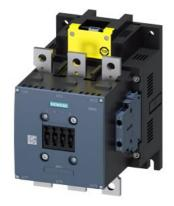
power contactor AC-1 400 A / 690 V / 40  $^{\circ}$ C 3-pole, Uc: 96-127 V AC(50-60 Hz) / DC F-PLC input 24 V DC drive: electronic auxiliary contacts 2 NO + 2 NC main circuit: busbar control and auxiliary circuit: screw terminal
