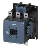
power contactor AC-1 400 A / 690 V / 40 °C 3-pole, Uc: 21-27.3 V AC(50-60 Hz) / DC PLC input 24 V DC drive: electronic auxiliary contacts 2 NO + 2 NC main circuit: busbar control and auxiliary circuit: screw terminal
