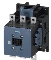
power contactor AC-1 400 A / 690 V / 40  $^\circ$ C 3-pole, Uc: 220-240 V AC(50-60 Hz) / DC drive: conventional auxiliary contacts 2 NO + 2 NC main circuit: busbar control and auxiliary circuit: screw terminal
