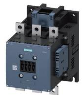
power contactor AC-1 400 A / 690 V / 40  $^\circ$ C 3-pole, Uc: 220-240 V AC(50-60 Hz) / DC drive: conventional auxiliary contacts 2 NO + 2 NC main circuit: busbar control and auxiliary circuit: spring-loaded terminal
