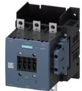
power contactor AC-1 275 A / 690 V / 40 °C 3-pole, drive: without auxiliary contacts 2 NO + 2 NC main circuit: busbar control and auxiliary circuit: screw terminal
