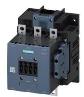
power contactor AC-1 275 A / 690 V / 40  $^\circ$ C 3-pole, Uc: 380-420 V AC(50-60 Hz) / DC drive: conventional auxiliary contacts 2 NO + 2 NC main circuit: busbar control and auxiliary circuit: screw terminal
