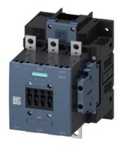
power contactor AC-1 275 A / 690 V / 40  $^{\circ}$ C 3-pole, Uc: 240-277 V AC(50-60 Hz) / DC drive: conventional auxiliary contacts 2 NO + 2 NC main circuit: busbar control and auxiliary circuit: screw terminal
