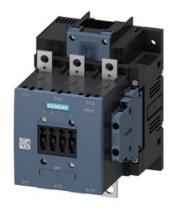
power contactor AC-1 275 A / 690 V / 40  $^{\circ}$ C 3-pole, Uc: 220-240 V AC(50-60 Hz) / DC drive: conventional auxiliary contacts 2 NO + 2 NC main circuit: busbar control and auxiliary circuit: screw terminal
