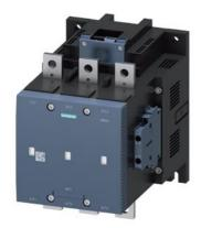
vacuum contactor AC-3e/AC-3 400 A, 200 kW / 400 V, 3-pole, Uc: 200-277 V AC(50-60 Hz) / DC PLC input 24 V DC drive: electronic auxiliary contacts 2 NO + 2 NC main circuit: busbar control and auxiliary circuit: screw terminal
