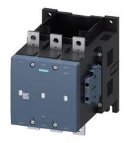
vacuum contactor AC-3e/AC-3 400 A, 200 kW / 400 V, 3-pole, Uc: 380-420 V AC(50-60 Hz) / DC drive: conventional auxiliary contacts 2 NO + 2 NC main circuit: busbar control and auxiliary circuit: screw terminal
