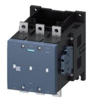
vacuum contactor AC-3e/AC-3 400 A, 200 kW / 400 V, 3-pole, Uc: 575-600 V AC(50-60 Hz) / DC drive: conventional auxiliary contacts 2 NO + 2 NC main circuit: busbar control and auxiliary circuit: screw terminal
