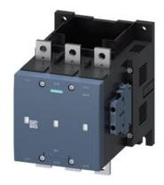
vacuum contactor AC-3e/AC-3 400 A, 200 kW / 400 V, 3-pole, Uc: 440-480 V AC(50-60 Hz) / DC drive: conventional auxiliary contacts 2 NO + 2 NC main circuit: busbar control and auxiliary circuit: screw terminal
