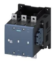
vacuum contactor AC-3e/AC-3 400 A, 200 kW / 400 V, 3-pole, Uc: 220-240 V AC(50-60 Hz) / DC drive: conventional auxiliary contacts 2 NO + 2 NC main circuit: busbar control and auxiliary circuit: screw terminal
