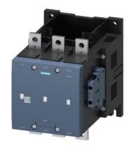
vacuum contactor AC-3e/AC-3 400 A, 200 kW / 400 V, 3-pole, Uc: 200-220 V AC(50-60 Hz) / DC drive: conventional auxiliary contacts 2 NO + 2 NC main circuit: busbar control and auxiliary circuit: screw terminal
