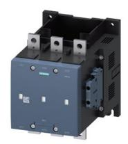
vacuum contactor AC-3e/AC-3 400 A, 200 kW / 400 V, 3-pole, Uc: 110-127 V AC(50-60 Hz) / DC drive: conventional auxiliary contacts 2 NO + 2 NC main circuit: busbar control and auxiliary circuit: screw terminal
