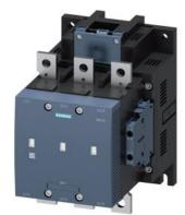
vacuum contactor AC-3e/AC-3 300 A, 160 kW / 400 V, 3-pole, Uc: 96-127 V AC(50-60 Hz) / DC PLC input 24 V DC drive: electronic auxiliary contacts 2 NO + 2 NC main circuit: busbar control and auxiliary circuit: screw terminal
