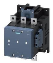
vacuum contactor AC-3e/AC-3 265 A, 132 kW / 400 V, 3-pole, Uc: 96-127 V AC(50-60 Hz) / DC PLC input 24 V DC drive: electronic auxiliary contacts 2 NO + 2 NC main circuit: busbar control and auxiliary circuit: screw terminal
