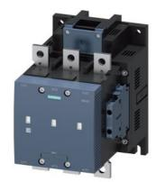
vacuum contactor AC-3e/AC-3 265 A, 132 kW / 400 V, 3-pole, Uc: 200-220 V AC(50-60 Hz) / DC drive: conventional auxiliary contacts 2 NO + 2 NC main circuit: busbar control and auxiliary circuit: screw terminal
