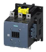
power contactor, AC-3e/AC-3 500 A, 250 kW / 400 V AC (50-60 Hz) / DC 200-277 V x (0.8-1.1) F-PLC input 24 V DC 3-pole, auxiliary contacts 2 NO + 2 NC drive: electronic main circuit: busbar control and auxiliary circuit: screw terminal
