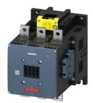
power contactor, AC-3e/AC-3 500 A, 250 kW / 400 V AC (50-60 Hz) / DC 200-277 V x (0.8-1.1) F-PLC input 24 V DC 3-pole, auxiliary contacts 2 NO + 2 NC permanently mounted drive: electronic main circuit: busbar control and auxiliary circuit: screw terminal
