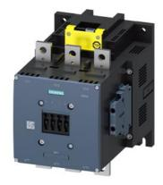
power contactor, AC-3e/AC-3 500 A, 250 kW / 400 V AC (50-60 Hz) / DC 96-127 V x (0.8-1.1) F-PLC input 24 V DC 3-pole, auxiliary contacts 2 NO + 2 NC drive: electronic main circuit: busbar control and auxiliary circuit: screw terminal
