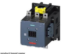
power contactor, AC-3e/AC-3 500 A, 250 kW / 400 V AC (50-60 Hz) / DC 96-127 V x (0.8-1.1) F-PLC input 24 V DC 3-pole, auxiliary contacts 2 NO + 2 NC permanently mounted drive: electronic main circuit: busbar control and auxiliary circuit: screw terminal
