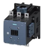
power contactor, AC-3e/AC-3 500 A, 250 kW / 400 V AC (50-60 Hz) / DC Uc: 200-277 V PLC input 24 V DC 3-pole, auxiliary contacts 2 NO + 2 NC drive: electronic main circuit: busbar control and auxiliary circuit: spring-loaded terminal
