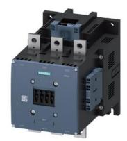
power contactor, AC-3e/AC-3 500 A, 250 kW / 400 V AC (50-60 Hz) / DC Uc: 96-127 V PLC input 24 V DC 3-pole, auxiliary contacts 2 NO + 2 NC drive: electronic main circuit: busbar control and auxiliary circuit: spring-loaded terminal
