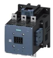
power contactor, AC-3e/AC-3 500 A, 250 kW / 400 V AC (50-60 Hz) / DC Uc: 21-27.3 V PLC input 24 V DC 3-pole, auxiliary contacts 2 NO + 2 NC drive: electronic main circuit: busbar control and auxiliary circuit: spring-loaded terminal
