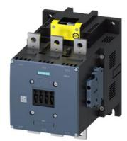
power contactor, AC-3e/AC-3 400 A, 200 kW / 400 V AC (50-60 Hz) / DC 96-127 V x (0.8-1.1) F-PLC input 24 V DC 3-pole, auxiliary contacts 2 NO + 2 NC drive: electronic main circuit: busbar control and auxiliary circuit: screw terminal
