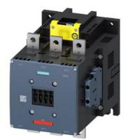
power contactor, AC-3e/AC-3 400 A, 200 kW / 400 V AC (50-60 Hz) / DC 96-127 V x (0.8-1.1) F-PLC input 24 V DC 3-pole, auxiliary contacts 2 NO + 2 NC permanently mounted drive: electronic main circuit: busbar control and auxiliary circuit: screw terminal
