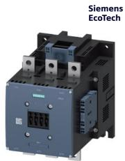
power contactor, AC-3e/AC-3 400 A, 200 kW / 400 V AC (50-60 Hz) / DC Uc: 220-240 V 3-pole, auxiliary contacts 2 NO + 2 NC drive: conventional main circuit: busbar control and auxiliary circuit: spring-loaded terminal
