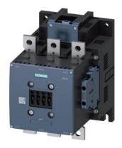
power contactor, AC-3e/AC-3 300 A, 160 kW / 400 V, Uc: 24 V DC x (0.7-1.25) PLC input 24-110 V DC 3-pole, auxiliary contacts 2 NO + 2 NC drive: electronic main circuit: busbar control and auxiliary circuit: screw terminal extended rated condition railroad IEC 60077
