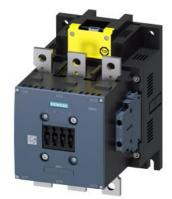
power contactor, AC-3e/AC-3 300 A, 160 kW / 400 V, AC (50-60 Hz) / DC 200-277 V x (0.8-1.1) F-PLC input 24 V DC 3-pole, auxiliary contacts 2 NO + 2 NC drive: electronic main circuit: busbar control and auxiliary circuit: screw terminal
