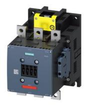
power contactor, AC-3e/AC-3 300 A, 160 kW / 400 V, AC (50-60 Hz) / DC 96-127 V x (0.8-1.1) F-PLC input 24 V DC 3-pole, auxiliary contacts 2 NO + 2 NC permanently mounted drive: electronic main circuit: busbar control and auxiliary circuit: screw terminal
