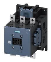
power contactor, AC-3e/AC-3 300 A, 160 kW / 400 V, AC (50-60 Hz) / DC Uc: 21-27, 3 V PLC input 24 V DC 3-pole, auxiliary contacts 2 NO + 2 NC drive: electronic main circuit: busbar control and auxiliary circuit: screw terminal
