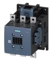
power contactor, AC-3e/AC-3 300 A, 160 kW / 400 V, AC (50-60 Hz) / DC Uc: 200-220 V 3-pole, auxiliary contacts 2 NO + 2 NC drive: conventional main circuit: busbar control and auxiliary circuit: screw terminal
