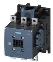
power contactor, AC-3e/AC-3 300 A, 160 kW / 400 V, AC (50-60 Hz) / DC Uc: 110-127 V 3-pole, auxiliary contacts 2 NO + 2 NC drive: conventional main circuit: busbar control and auxiliary circuit: screw terminal
