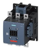
power contactor, AC-3e/AC-3 300 A, 160 kW / 400 V, AC (50-60 Hz) / DC Uc: 23-26 V 3-pole, auxiliary contacts 2 NO + 2 NC permanently mounted drive: conventional main circuit: busbar control and auxiliary circuit: screw terminal
