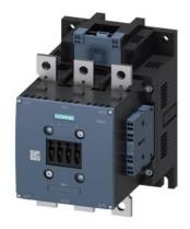
power contactor, AC-3e/AC-3 300 A, 160 kW / 400 V, Uc: 24 V DC x (0.7-1.25) PLC input 24-110 V DC 3-pole, auxiliary contacts 2 NO + 2 NC drive: electronic main circuit: busbar control and auxiliary circuit: spring-loaded terminal extended rated condition railroad IEC 60077
