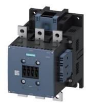
power contactor, AC-3e/AC-3 300 A, 160 kW / 400 V, AC (50-60 Hz) / DC Uc: 110-127 V 3-pole, auxiliary contacts 2 NO + 2 NC drive: conventional main circuit: busbar control and auxiliary circuit: spring-loaded terminal
