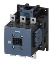
power contactor, AC-3e/AC-3 300 A, 160 kW / 400 V, AC (50-60 Hz) / DC Uc: 23-26 V 3-pole, auxiliary contacts 2 NO + 2 NC drive: conventional main circuit: busbar control and auxiliary circuit: spring-loaded terminal
