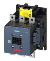
power contactor, AC-3e/AC-3 265 A, 132 kW / 400 V AC (50-60 Hz) / DC 200-277 V x (0.8-1.1) F-PLC input 24 V DC 3-pole, auxiliary contacts 2 NO + 2 NC permanently mounted drive: electronic main circuit: busbar control and auxiliary circuit: screw terminal
