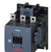
power contactor, AC-3e/AC-3 265 A, 132 kW / 400 V AC (50-60 Hz) / DC Uc: 200-277 V PLC input 24 V DC 3-pole, auxiliary contacts 2 NO + 2 NC permanently mounted drive: electronic main circuit: busbar control and auxiliary circuit: screw terminal
