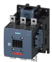
power contactor, AC-3e/AC-3 265 A, 132 kW / 400 V AC (50-60 Hz) / DC Uc: 110-127 V 3-pole, auxiliary contacts 2 NO + 2 NC permanently mounted drive: conventional main circuit: busbar control and auxiliary circuit: screw terminal
