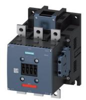
power contactor, AC-3e/AC-3 265 A, 132 kW / 400 V AC (50-60 Hz) / DC Uc: 23-26 V 3-pole, auxiliary contacts 2 NO + 2 NC permanently mounted drive: conventional main circuit: busbar control and auxiliary circuit: screw terminal
