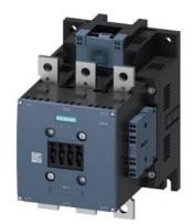
power contactor, AC-3e/AC-3 265 A, 132 kW / 400 V AC (50-60 Hz) / DC Uc: 96-127 V PLC input 24 V DC 3-pole, auxiliary contacts 2 NO + 2 NC drive: electronic main circuit: busbar control and auxiliary circuit: spring-loaded terminal
