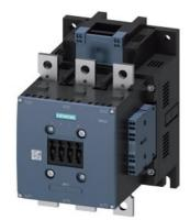
power contactor, AC-3e/AC-3 265 A, 132 kW / 400 V AC (50-60 Hz) / DC Uc: 440-480 V 3-pole, auxiliary contacts 2 NO + 2 NC drive: conventional main circuit: busbar control and auxiliary circuit: spring-loaded terminal
