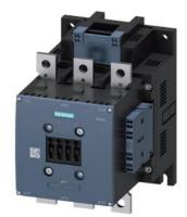
power contactor, AC-3e/AC-3 265 A, 132 kW / 400 V AC (50-60 Hz) / DC Uc: 110-127 V 3-pole, auxiliary contacts 2 NO + 2 NC drive: conventional main circuit: busbar control and auxiliary circuit: spring-loaded terminal
