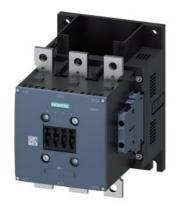
power contactor, AC-3e/AC-3 225 A, 110 kW / 400 V without operating mechanism 3-pole, auxiliary contacts 2 NO + 2 NC main circuit: busbar control and auxiliary circuit: screw terminal
