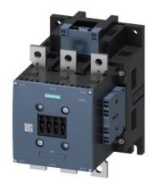
power contactor, AC-3e/AC-3 225 A, 110 kW / 400 V AC (50-60 Hz) / DC Uc: 21-27, 3 V PLC input 24 V DC 3-pole, auxiliary contacts 2 NO + 2 NC drive: electronic main circuit: busbar control and auxiliary circuit: spring-loaded terminal
