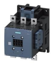
power contactor, AC-3e/AC-3 225 A, 110 kW / 400 V AC (50-60 Hz) / DC Uc: 240-277 V 3-pole, auxiliary contacts 2 NO + 2 NC drive: conventional main circuit: busbar control and auxiliary circuit: spring-loaded terminal
