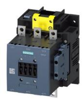
power contactor, AC-3e/AC-3 185 A, 90 kW / 400 V AC (50-60 Hz) / DC Uc: 200-277 V x (0.8-1.1) F-PLC input 24 V DC 3-pole, auxiliary contacts 2 NO + 2 NC drive: electronic main circuit: busbar control and auxiliary circuit: screw terminal
