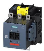
power contactor, AC-3e/AC-3 185 A, 90 kW / 400 V AC (50-60 Hz) / DC Uc: 200-277 V x (0.8-1.1) F-PLC input 24 V DC 3-pole, auxiliary contacts 2 NO + 2 NC permanently mounted drive: electronic main circuit: busbar control and auxiliary circuit: screw terminal
